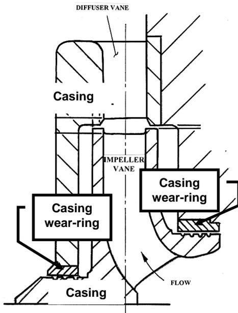
Figure 2 – Impeller Wear-Rings
