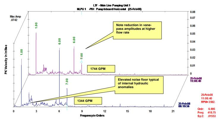
Figure 8 - PIH spectra at different flow rates exemplifying the reduction of vane-pass amplitudes at higher flow rate
