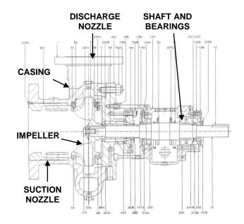
Figure 1 – Typical Centrifugal Pump
