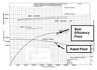
Figure 3 – Typical Pump Characteristic Curves
