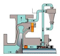
Figure 9 – API Seal Flush Plan 31 with Cyclone Separator
