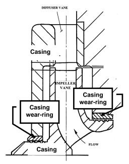
Figure 2 – Impeller Wear-Rings
