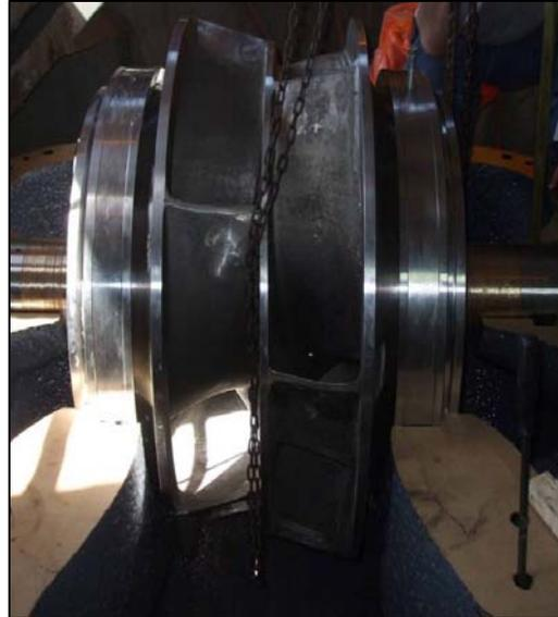
FIGURE 12: REPLICATED IMPELLER
