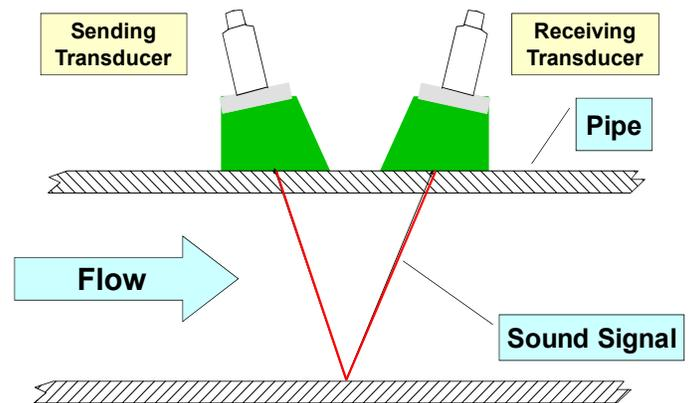
**FIGURE 4: TWO PASS ULTRASONIC FLOW MEASUREMENT
